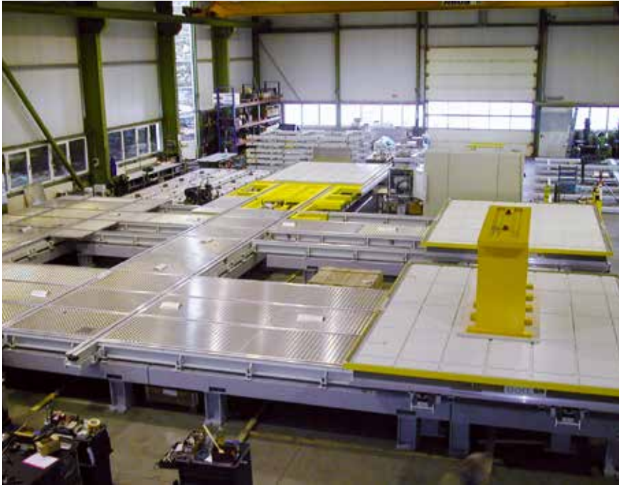
Workpiece serving and storage system (horizontal) Pallet size 3200 × 4200 mm
